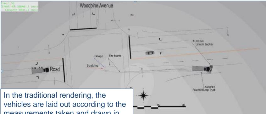
vehicles are laid out according to the measurements taken and drawn in reference to the related items. This was usually done on site. Much time was needed for this.
